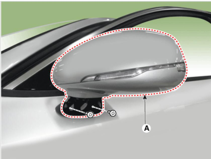
3. Remove the outside rear view mirror after disconnecting the connector (A).
